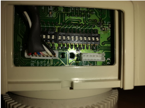
FIGURE 4.20: AS20RS485 dip-switches selection for Pelco-P
