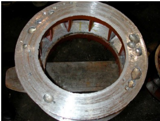
FIGURE 3.1: Severe case of porosity in the end ring of the aluminum casted rotor cage [44]
