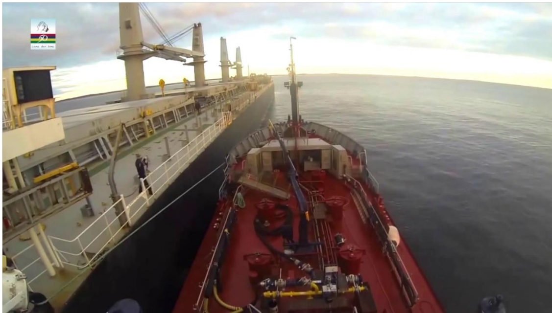
Figure II-E: The bunker tanker is berthed onto the receiving vessel.
