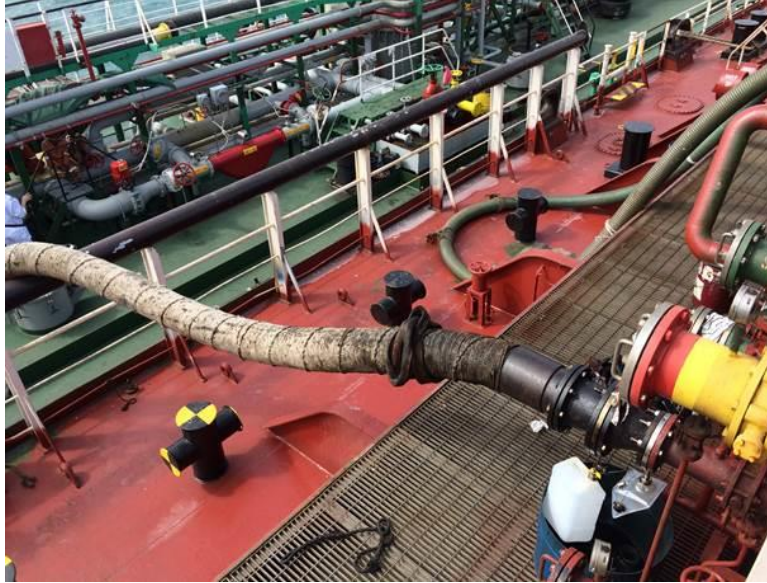
Figure II-F: The bunkering hose is connected to the vessel's manifold
