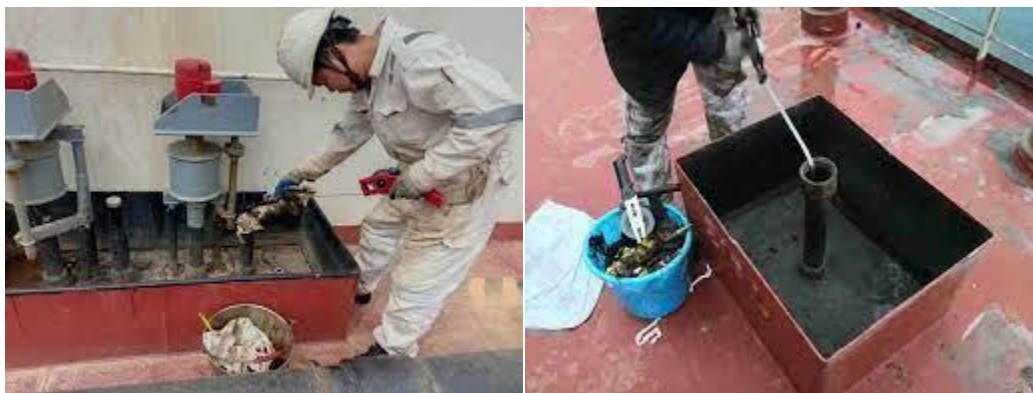
Figure II-H: Personnel sounding a tank
