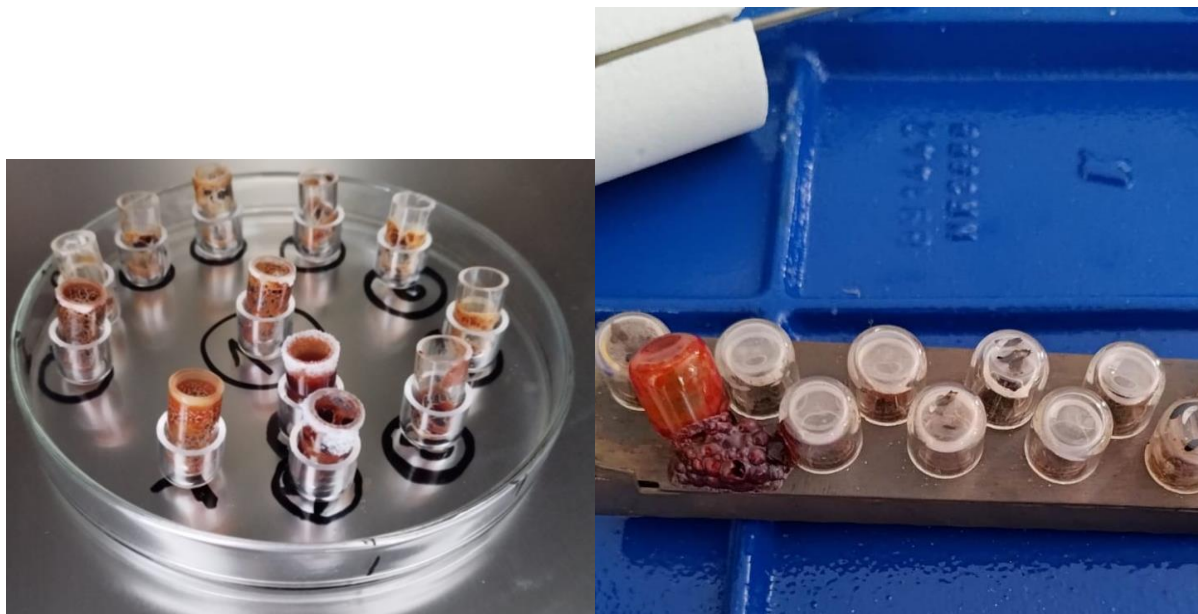
Pic.8.3.1: Crucibles with different undesirable outcomes.
