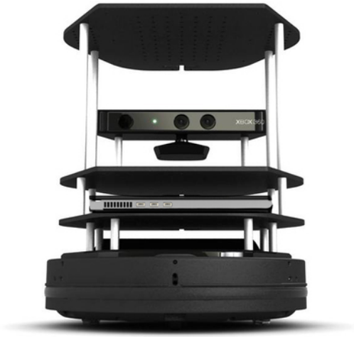
(a) The Default Configuration of the Turtlebot2 Platform.
