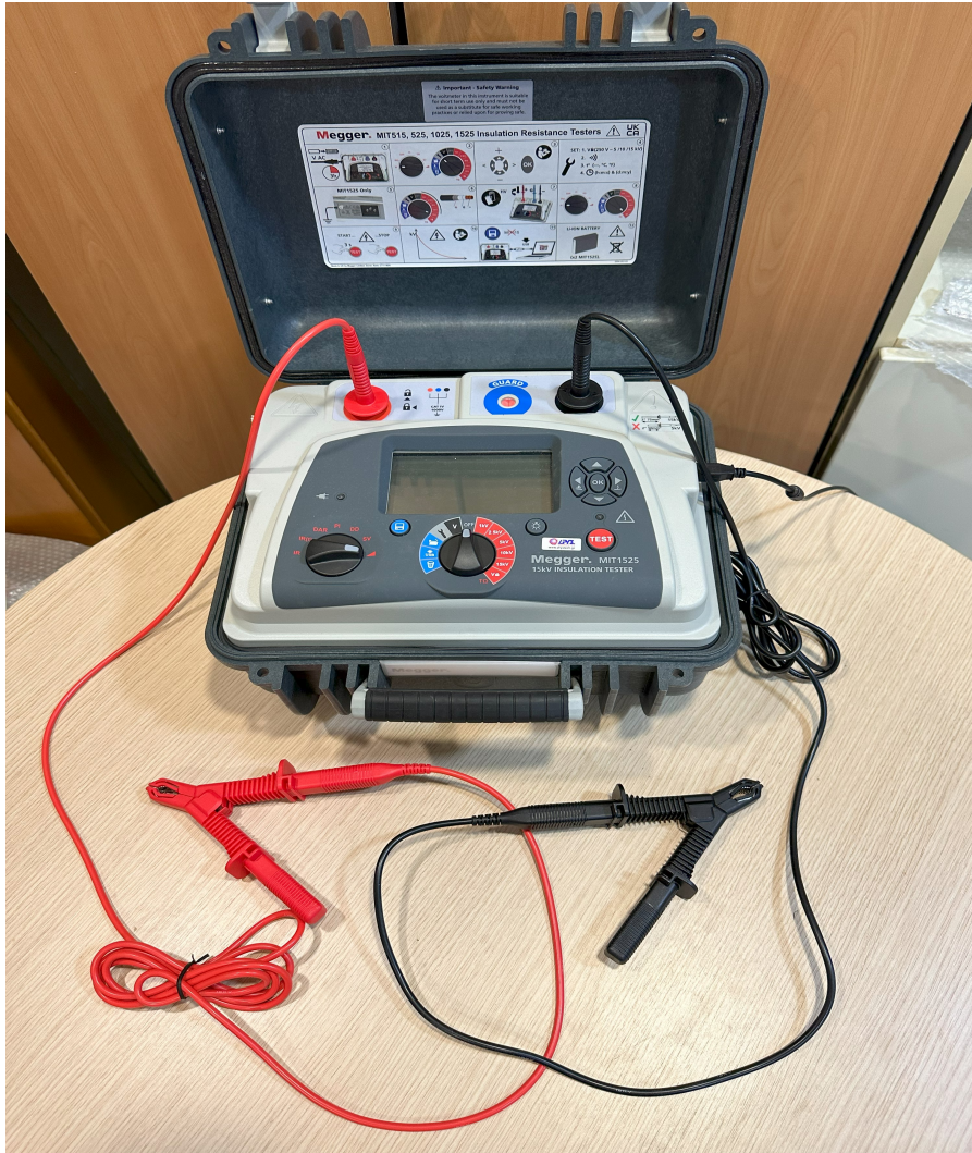
Figure 4.15: The Megger MIT1525 15kV instrument in the lab with clamps connected to the positive (red) and negative (black) terminals
