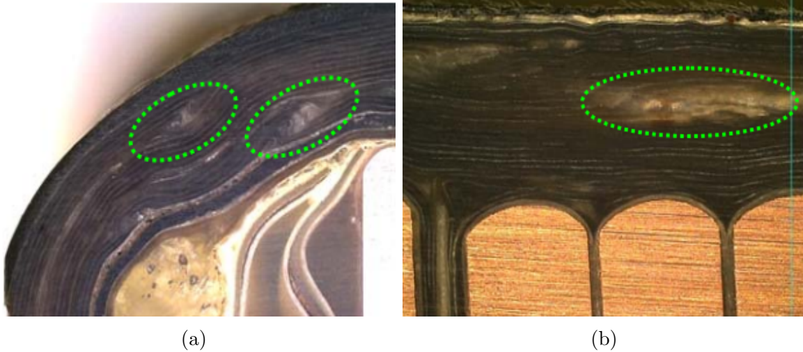
Figure 3.3: Coil cross section showing tape damage before applied to the coil [73]
