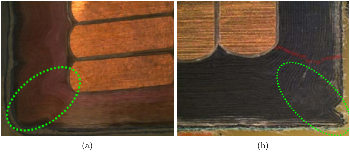
Figure 3.6: Coil cross section showing sharp edges [73]
