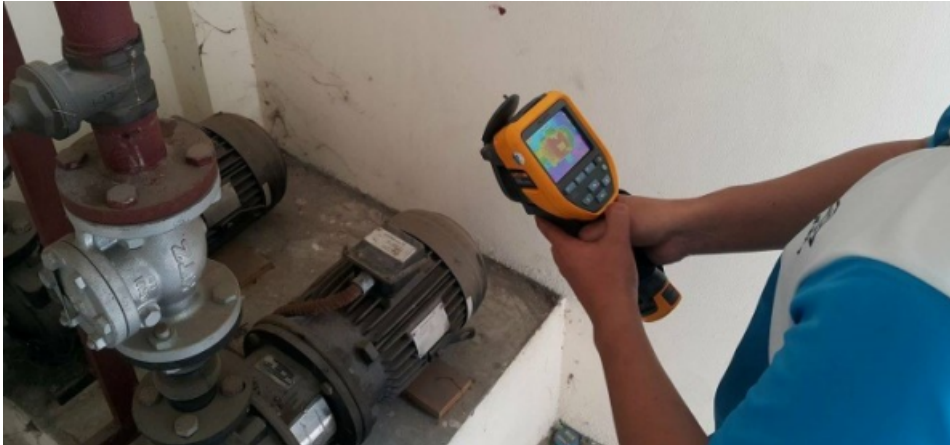
Figure 2.7: Examining a motor with thermography [64]
