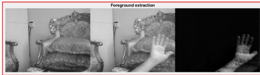
Image 4: Foreground extraction is used in appearance recognition to isolate the Region of Interest (ROI), utilizing techniques such as pattern subtraction and foreground segmentation algorithms.
