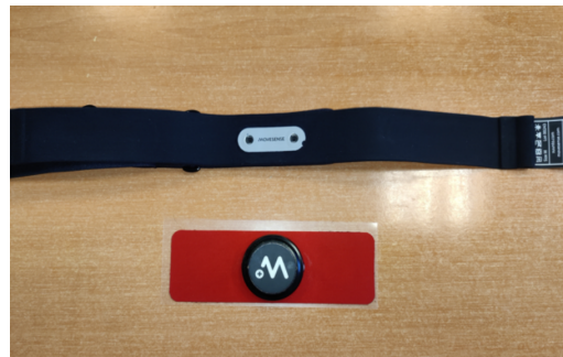
FIGURE 4.14: The multisensory device Movesense Medical is attached to an electrode (bottom) and the chest belt used (top).
