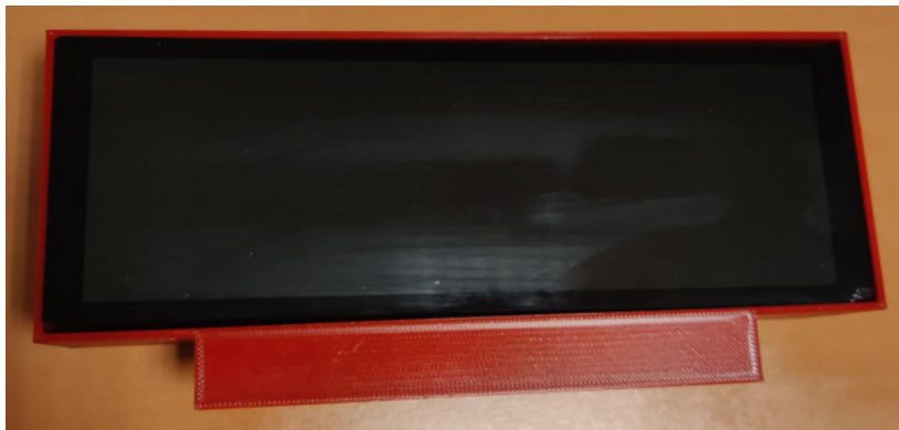
FIGURE 4.17: The 3d case hosting the raspberry unit attached to the monitor.
