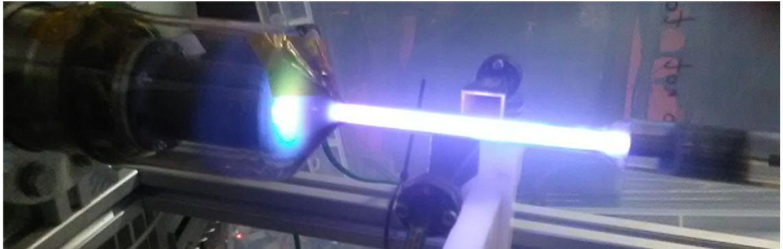
Figure 3.2: Hollow-Cathode plasma discharger
