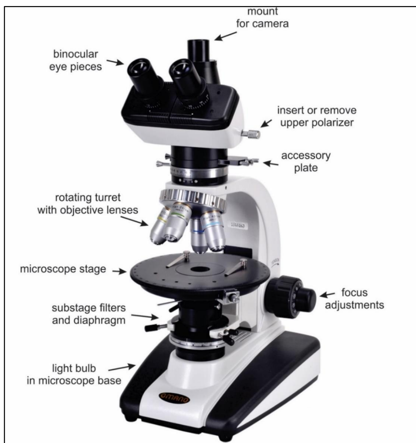
Figure 8: The components of a conventional optical microscope (OM) used for rocks and minerals observation (aka petrographic microscope). Image Source: https://opengeology.org/Mineralogy/5-optical-mineralogy
