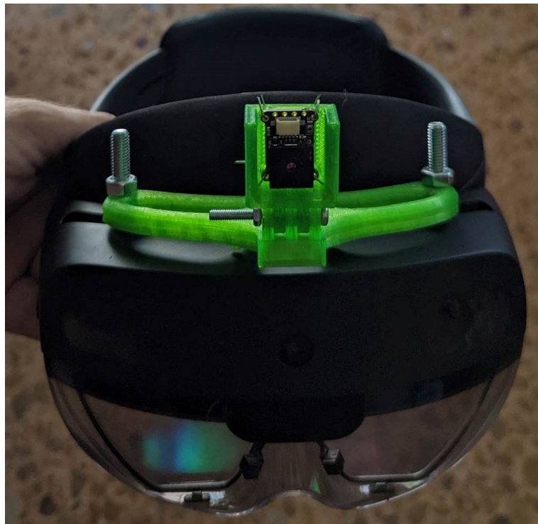
Figure 5.2: FLIR thermal camera mounted on top of the HoloLens 2
