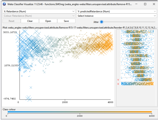
Figure 4.7: SMOREg Classifier Errors. Actual retardance (x axis) vs predicted Retardance (y axis).
