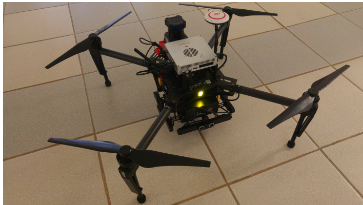
Figure 2.5: The DJI M100 quadcopter equipped with the Manifold unit, a LiDAR sensor and the Guidance system.
