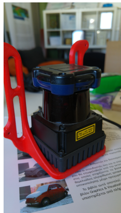
(a) The LiDAR Hokuyo UTM-30LX-EW
