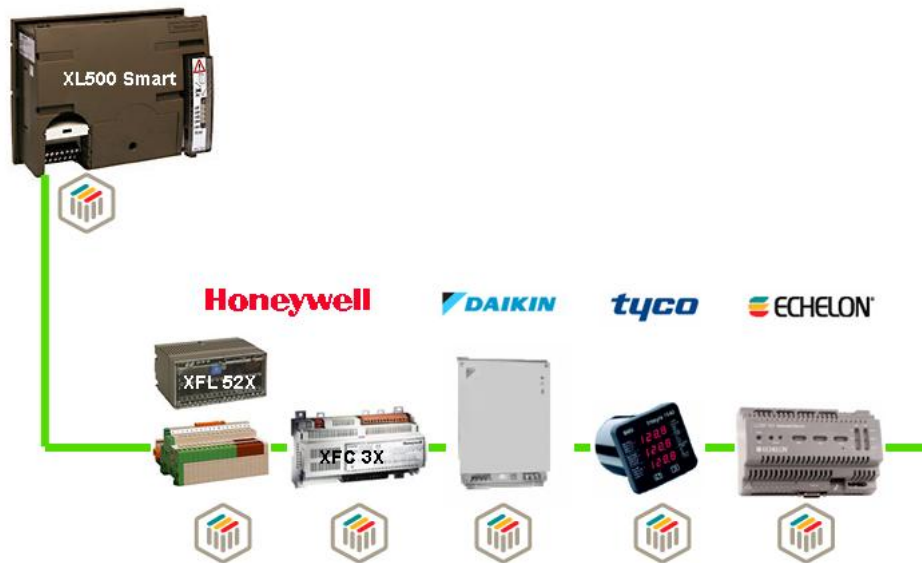
Figure 4-8: The Lonworks control network.
