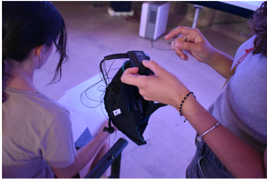
(a) EEG headset preparation with conductive gel application
