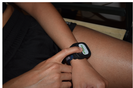
(b) Placement of the Traqbeat wrist monitor on the participant's dominant wrist for backup heart rate monitoring.
