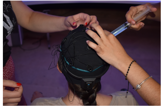
(b) Headset positioning and electrode adjustment
