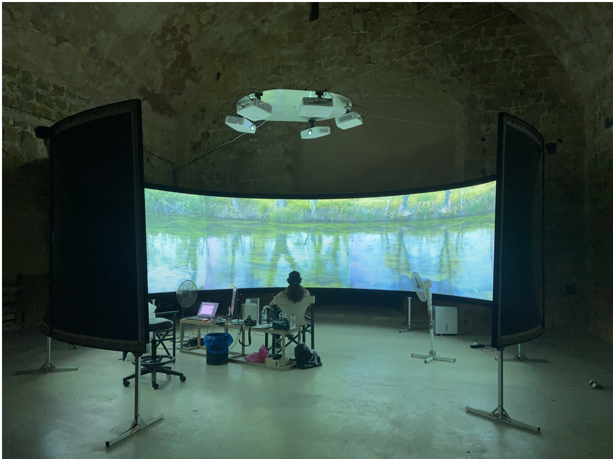
Figure 3.12: Experimental setup along with the participant seated at the center with EEG and ECG devices.
