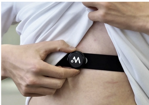
(a) Placement of the Movesense ECG chest strap on the participant's torso for primary cardiac signal recording.
