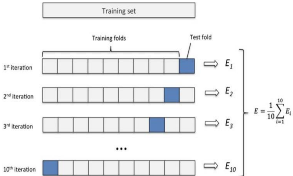
Figure 4.43: Diagram of k -fold cross-validation, where k=10 [97]
