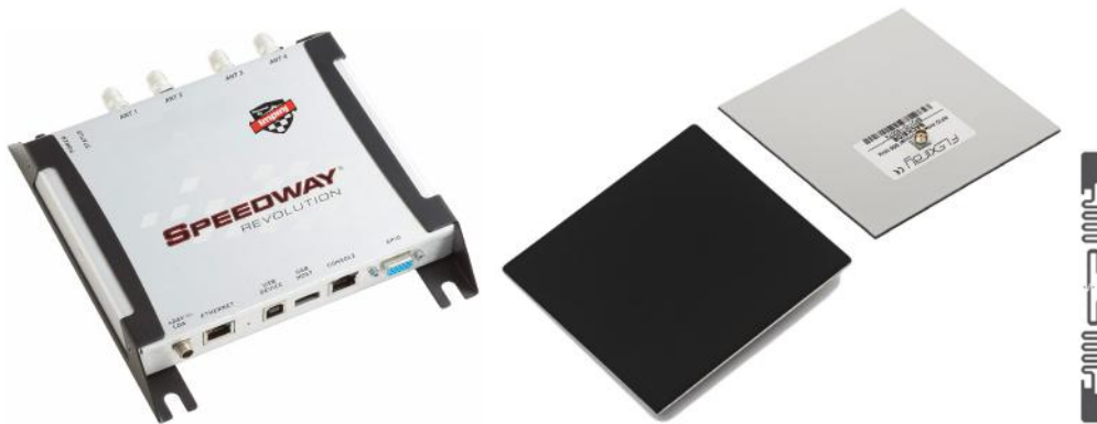
Figure 1.2: RFID reader (left), antennas (middle) and passive tag (right)
