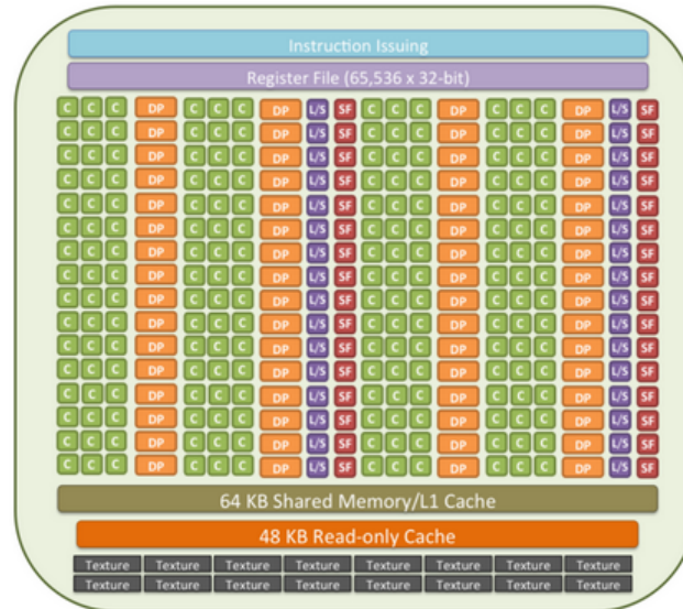
FIGURE 2.3: GPU Streaming multiprocessor's architecture
